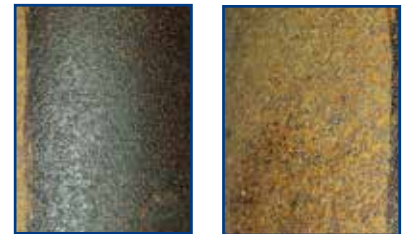
with Rust Converter without Rust Converter
